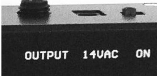
The Miami has an On/Off slide switch on the right side of the rear panel. Replacement AC Adapters can be ordered from [acidlab.de](http://acidlab.de) .
