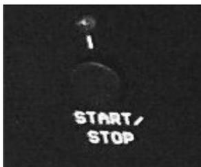
The Start/Stop button works in every mode and returns the pattern to its starting point, i.e. step 1 of the current pattern.
