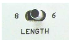
With the length switch the step length of the external synchronisation can be changed (triole if on 8; 1/16 if on 6).
