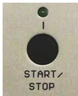
You can adjust the tempo with the Tempo Knob, and the Start/Stop button will start or stop the sequencer.
