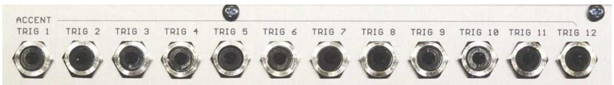
Every trigger-output without programmed Accent on this step has an amplitude of 4,2 Volt, and the duration of the impulse is 10ms.
