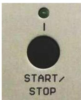
The Start/Stop button works in every mode and returns the pattern to its starting point, i.e. step 1 of the current pattern.
