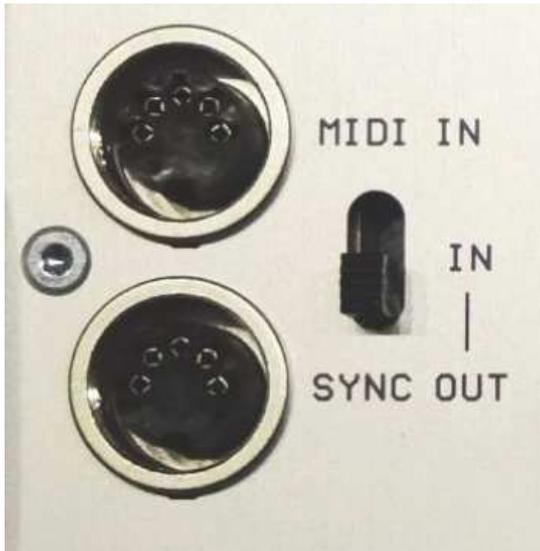
A Sync-out Signal will be generated at the Sync socket for other devices that have a Sync-In socket.
