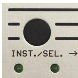
If the Clear Button and the Inst./Select button are held for a longer period, all triggers will be erased from the steps the sequencer passes through during the time the buttons are held.
