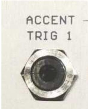
The Accent-/Trig1 Out is primarily intended to be used to control a Trigger- or Accent In of any drum-module or gate-/trigger input of an analog synthesizer, or any other event in your modular system.
