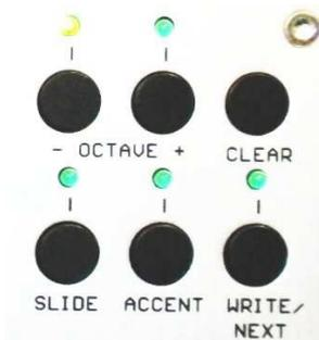
The LEDs over the buttons indicate the programming of Slide, Accent, Oktave Up/Down on the active note.
