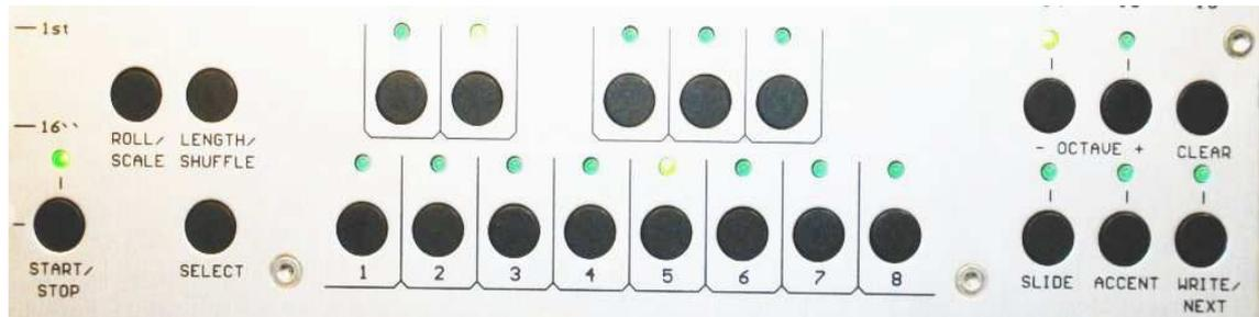
With pressing one of the buttons 1-8 of the keyboard, the step is directly selected e.g. the step 7. Now this step can be changed.
