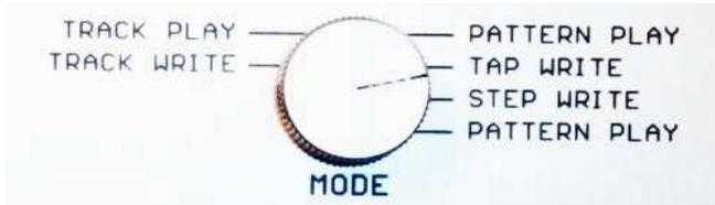
In all six modes the playing of the sequencer is guaranteed. You can change the modes, while the sequencer is running. Switching into another mode, takes place after the last step of the current pattern.
