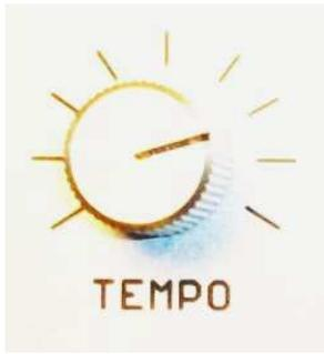
With Tempo, the speed of the internal clock generator is controlled.
