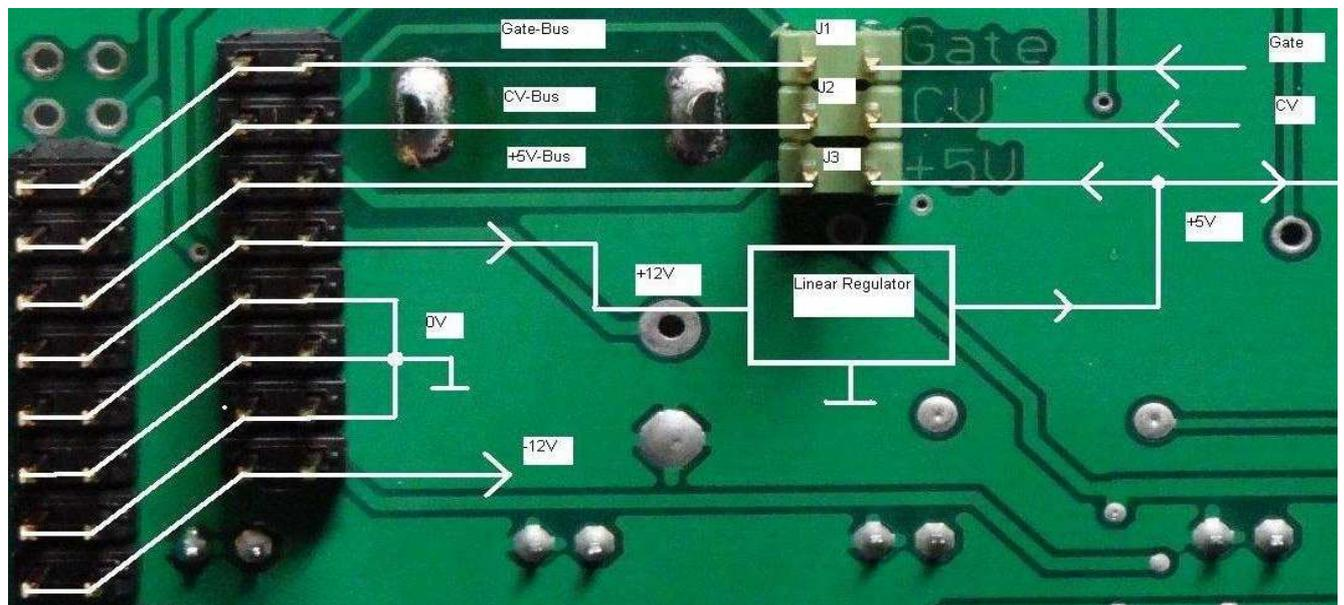
***The +5V supply of the Autobot can be loaded up to 200mA.***
