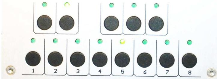
With the pressing of a button of the keyboard, you set a note with the corresponding pitch on the step. By continuous pressing of a button, this corresponding note is programmed on several steps. You can add Accent, Slide and Octave Up/Down with the corresponding buttons to the programmed notes.
