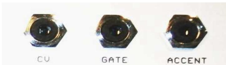
Over the sockets CV Out and Gate Out (3.5 mm, mono) compatible synthesizers can be played. CV Out is a 1V/Oktave control voltage for the pitch, and Gate Out and Accent Out are +12V impulses with the note length information.
