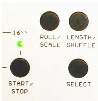
Start/Stop works in each mode, and puts the pattern back to the starting point step 1 of the current pattern.
