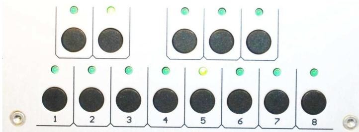
The current pattern is indicated with the LEDs 1-8. A pattern consists of maximally 16 steps.
