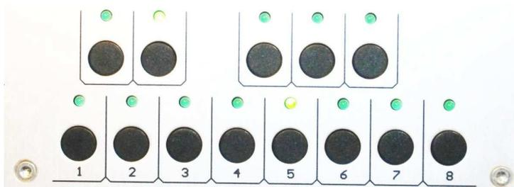
The active pattern is indicated with the LED over the button and is played repetitive. Press Write/Next and the current pattern becomes the first pattern of the track.
