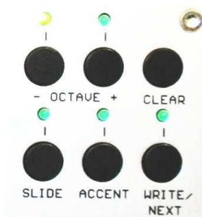
Press the button Write/Next again, and the step 3 is shown, etc.. After the last step of the patterns (dependent on the pattern length programming) the cursor jumps back on step 1.
