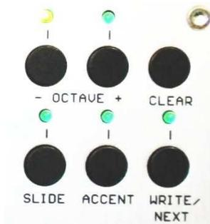
Then a new Pattern can be selected. Press the Write/Next button, and the second Pattern is fixed in the TRACK. The selected Pattern is sequentially repeated as in the Pattern Play mode. As in the Pattern Play mode you can chain several Pattern and be written with a Write/Next completely in the track.
