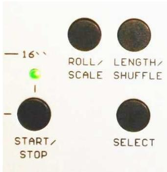
The selected step and its cursor is shifted to the left when you press the bottom Roll.
