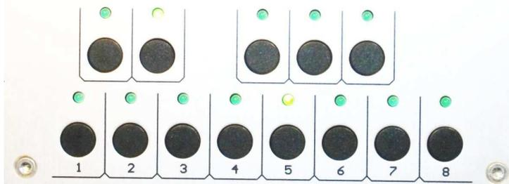
LEDs 1-4 of the step buttons will now indicate the shuffle setting of the first kind of shuffle.
