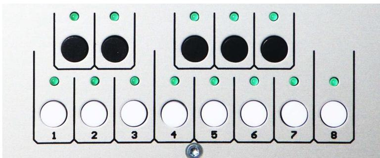
With the pressing of a button of the keyboard, you set a note with the corresponding pitch on the step. By continuous pressing of a button, this corresponding note is programmed on several steps. You can add Accent, Slide and Octave Up/Down with the corresponding buttons to the programmed notes.
