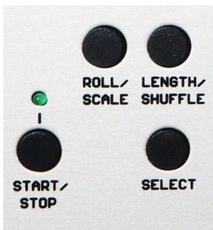
Start/Stop works in each mode, and puts the pattern back to the starting point step 1 of the current pattern.
