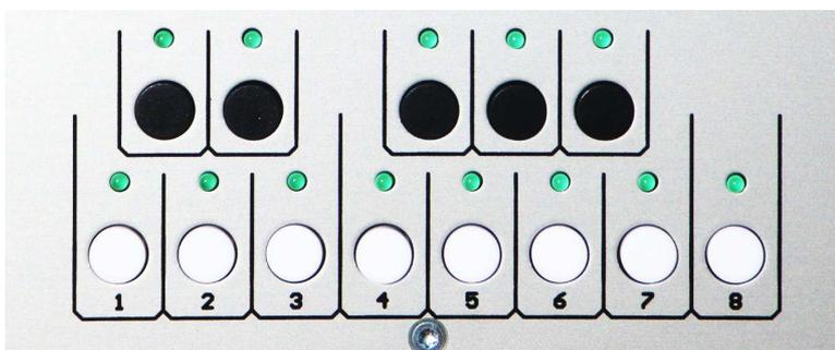
The active pattern is indicated with a flashing LED over the button. When pressing a new pattern, this LED lights continuously. After the pattern changed after the last step, to selected pattern, this LED flashes again.
