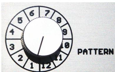
The pattern is selected from one of the 12 pattern groups. You can change the pattern group at all times with the rotary switch, and the switching into the new pattern group takes place after the last step of the current pattern.
