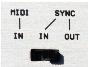
At the Sync socket there is a Sync Out signal that can be used to synchronise other gear with Sync In.
