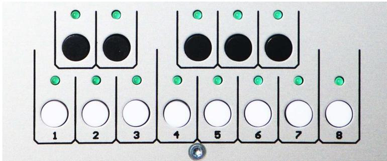
The current pattern is indicated with the LEDs 1-8. A pattern consists of maximally 16 steps.
