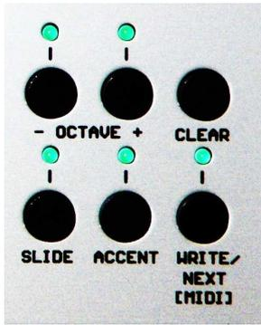
The LEDs over the keys indicate the programming of Octave Up/Down, Slide, Accent, of the note.
