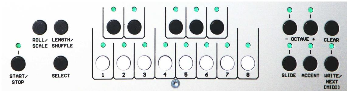
With pressing one of the buttons 1-8 of the keyboard, the step is directly selected e.g. the step 7. Now this step can be changed.
