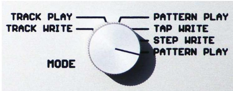
In all six modes the playing of the sequencer is guaranteed. You can change the modes, while the sequencer is running. Switching into another mode, takes place after the last step of the current pattern.
