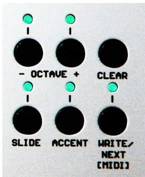
Press the button Write/Next again, and the step 3 is shown, etc.. After the last step of the patterns (dependent on the pattern length programming) the cursor jumps back on step 1.
