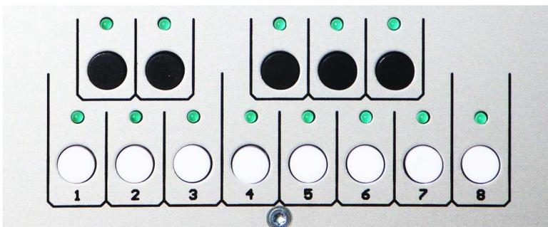
The active pattern is indicated with the LED over the button and is played repetitive. Press Write/Next and the current pattern becomes the first pattern of the track.
