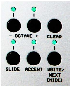
Then a new Pattern can be selected. Press the Write/Next button, and the second Pattern is fixed in the TRACK. The selected Pattern is sequentially repeated as in the Pattern Play mode. As in the Pattern Play mode you can chain several Pattern and be written with a Write/Next completely in the track.
