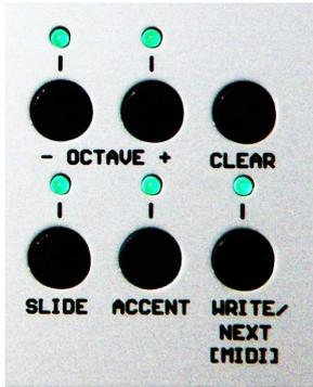
The LEDs over the buttons indicate the programming of Slide, Accent, Oktave Up/Down on the active note.
