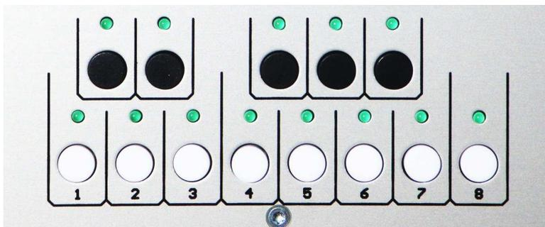
LEDs 1-4 of the step buttons will now indicate the shuffle setting of the first kind of shuffle.
