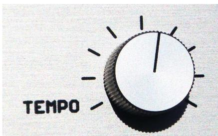
With Tempo, the speed of the internal clock generator is controlled.
