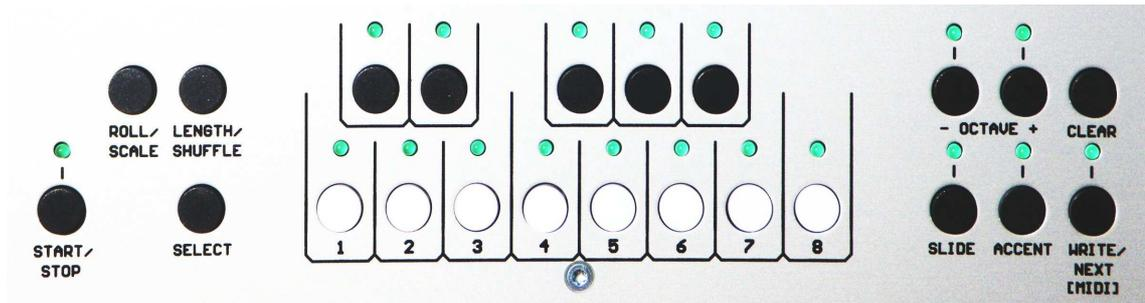
Now the entire pattern is transposed by the pitch offset that has been added. This transposed pattern repeats and can be changed with the repeated pressing of the Select button and a new pitch offset again. This new, transposed pattern, can be programmed like the other patterns, with the Write/Next button into the Track.
